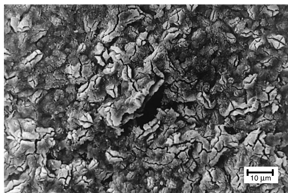
Fig. 4. SEM micrographs of niobium oxide film growth in 0.1 \text{ M H}_2\text{C}_2\text{O}_4 with i = 8 \text{ mA cm}^{-2} , Nb electrode polarized for 2300 s with a final potential of 100 V after successive breakdowns.
